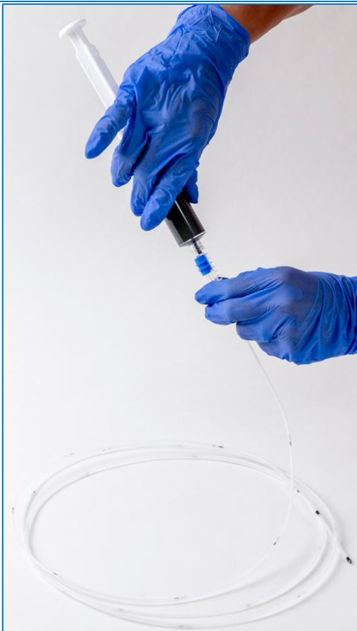
Fig. 18 Connecting the syringe to the EV valve.
