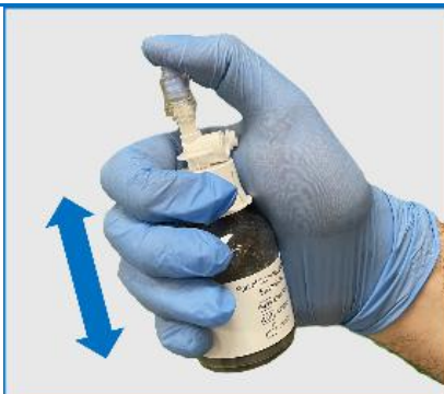
Fig. 14 Shaking vertically for 5 seconds.
