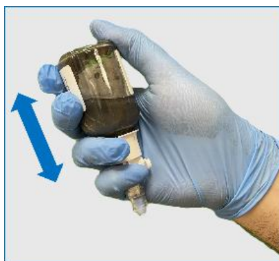
Fig. 15 Turning the components 180° and shaking vertically for 5 seconds.
