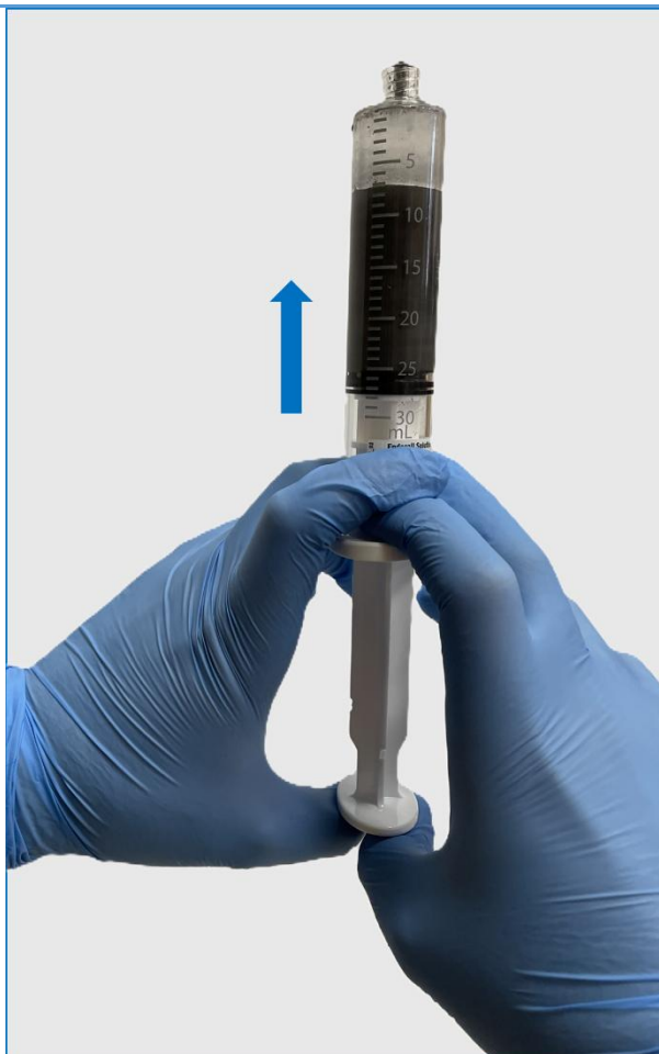
Fig. 22 Removing air from the syringe.
